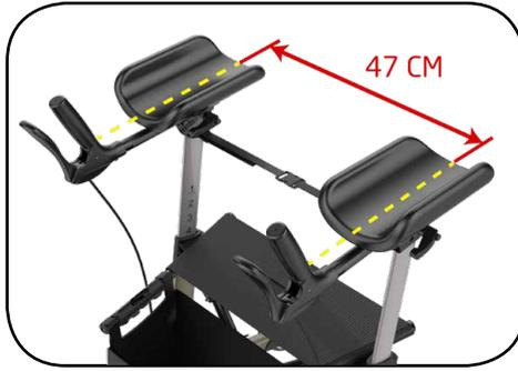
Centre-to-centre distance between forearm supports is 47 cm. It is equipped with a strap in order to stabilize and strengthen the upper part. The strap must be connected during use.
