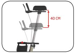
The height adjustable forearm supports are very easy to adjust in a range of 75 - 115 cm (total for both rollator sizes).
