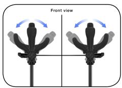
The push handles can be rotated to fit the most comfortable position of the user's hand. Width between push handles is 47 cm.
