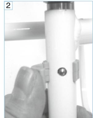
Put the premounted backrest on the basic rack and fix it with the star screws with a clockwise rotation. (See picture 3).
