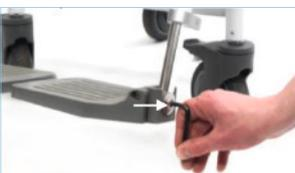
To adjust the footplate angle, slacken the bolt near the bottom of the inner tube (chrome). Adjust the footplate to the required angle and resecure the bolt.
