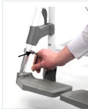
To adjust the height of the footplate, slacken the bolt at the end of the white tubing of the leg rest, using an allen key and turning the bolt anticlockwise. Slide the footrest to the required height and secure the footrest by retightening the bolt. Tighten the bolt by turning clockwise with an allen key
